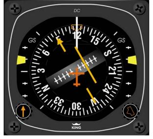
The more the CDI moves to the center, the more the aircraft has to be steered to the left in order to hold the CDI under the lubber line. The best way is to position the end of the CDI needle under the lubber line. This way the angle between the HSI arrow-head
