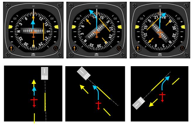
When the CDI starts moving away from the instrument edge, the aircraft is 2.5° away from the localizer centerline.
