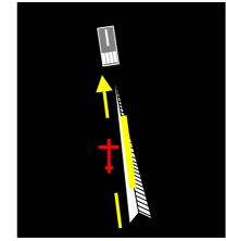
The CDI is located ahead of the aircraft, which means the aircraft flies towards the localizer.
