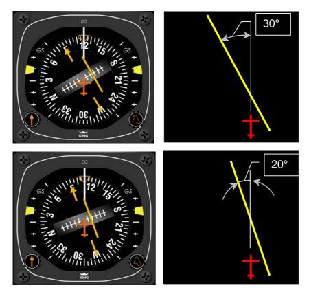
The aircraft intercepts the localizer with an angle of 30°.
