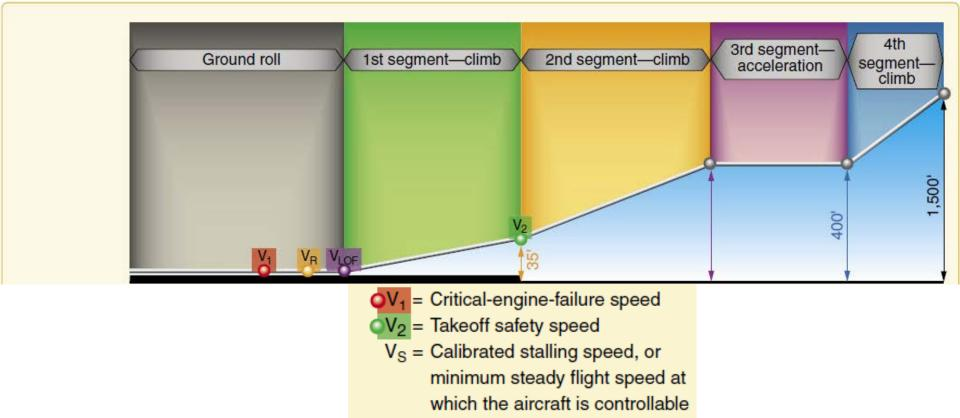
V<sub>R</sub> = Speed at which aircraft can
