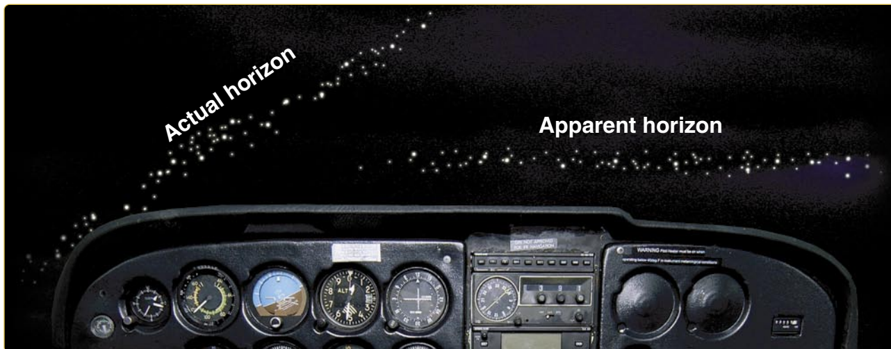
Figure 16-15. At night, the horizon may be hard to discern due to dark terrain and misleading light patterns on the ground.
