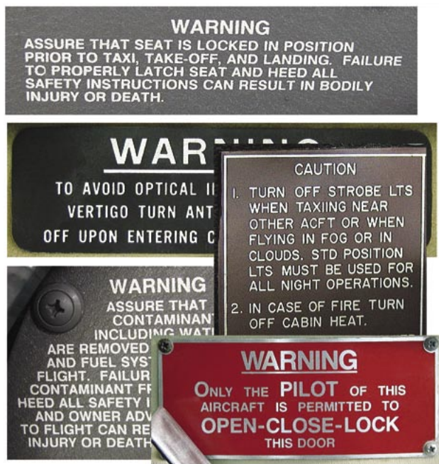
Figure 8-5. Placards are used to depict aircraft limitations.
