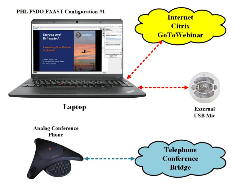
This Visio schematic illustrates another alternative for the PHL FSDO FAAST presenter's configuration. This configuration would be useful when the FAAST member delivering the presentation is at one location and the supporting FAAST members are at the other locations. The author of this article would use the aviation headset connected to the iPhone via Bluetooth.
