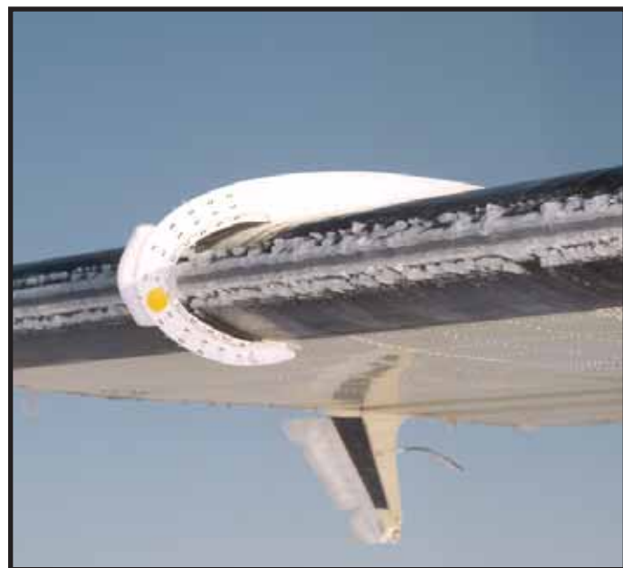
Mixed ice formation on wing leading edge
