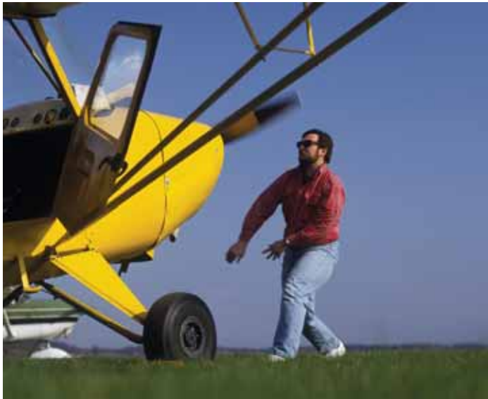
Do not attempt hand-propping without proper training.
