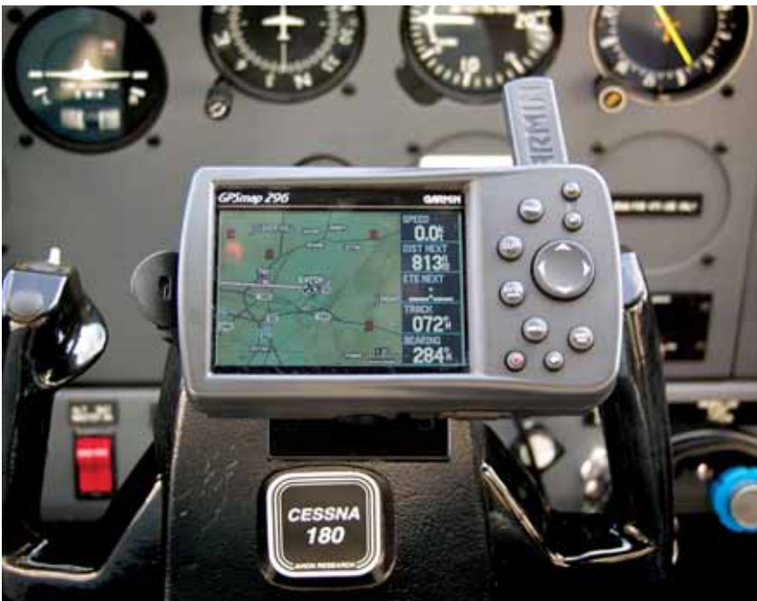
Although not legal for navigation under IFR, a hand-held or yoke-mounted GPS receiver can be useful in maintaining situational awareness.
