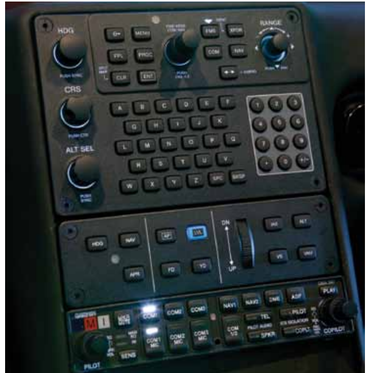
Recent trends toward larger, FMS-style keyboards (and fewer multifunction keys) hold promise for easier data entry and quicker transitions to new equipment.
