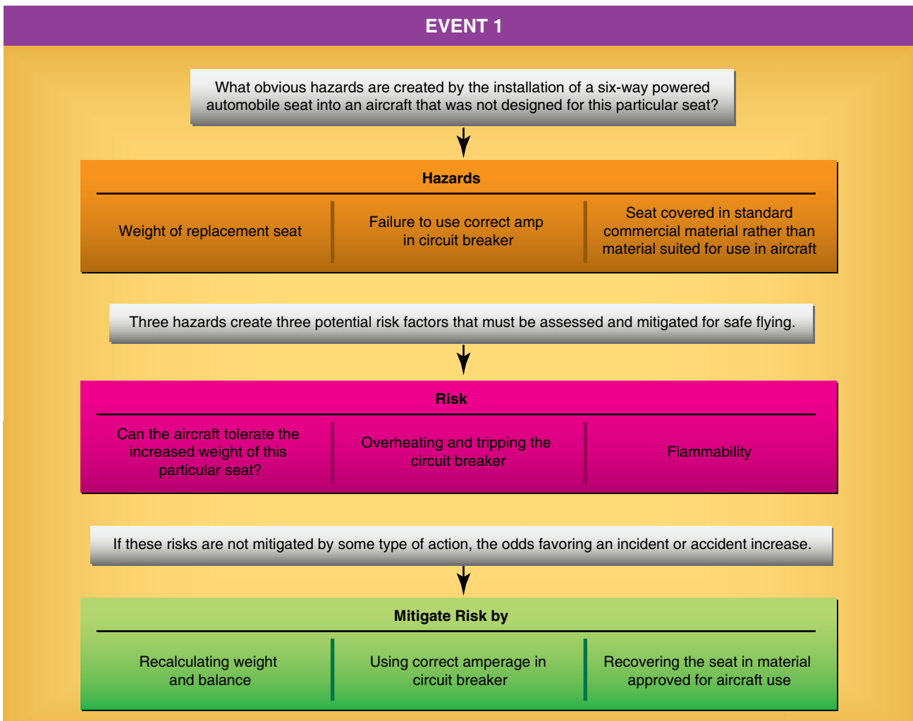
Figure 6-4. Example of an event diagram mapping hazards, risk assessment, and risk mitigation for the first event.
