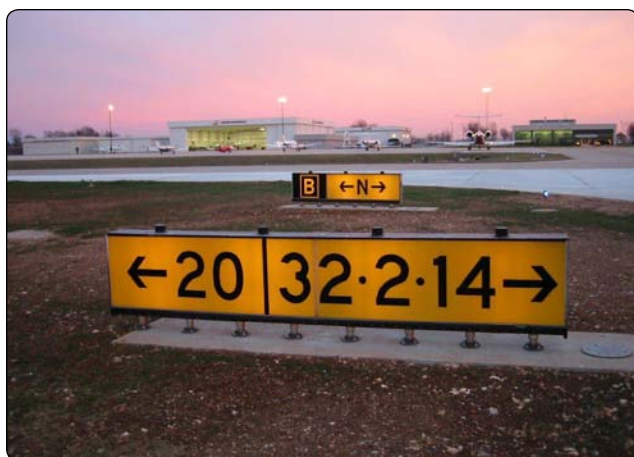
Figure 1-35. Runway destination sign with different taxi routes.
