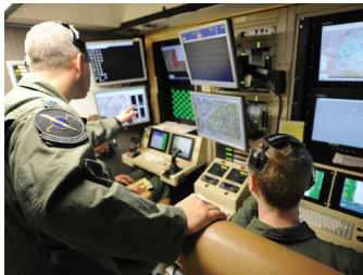
A VIEW INSIDE THE GROUND CONTROL STATION OF AN MQ-9 DURING A TRAINING MISSION.
