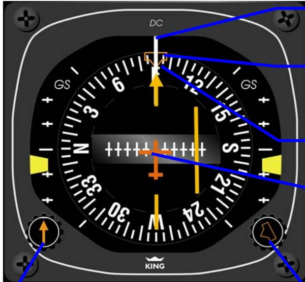
The **lubber line** defines the aircrafts longitudinal axis.
