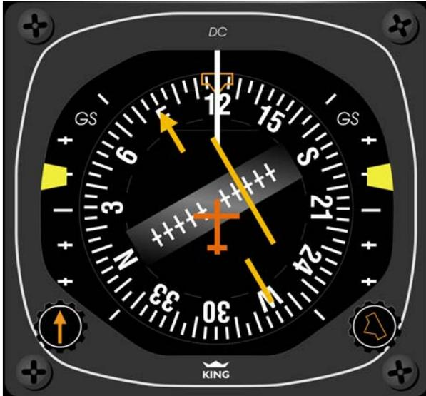
The best way is to position the end of the CDI needle under the lubber line. This way the angle between the HSI arrow-head (course pointer) and the lubber line will be your interception angle.
